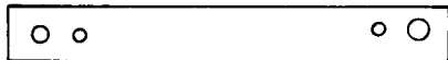
Q202—RIBBON, SHORT \frac{3}{8} " x .004 x 2 \frac{3}{4} " cc large holes \frac{3}{8} " x .004 x 2- \frac{3}{16} " cc small holes (3- \frac{3}{16} " long, also carried in .003)
