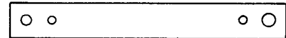
Q201—RIBBON \frac{3}{8} " x .004 x 2- \frac{13}{16} " cc large holes \frac{3}{8} " x .004 x 2- \frac{9}{32} " cc small holes (3 \frac{1}{4} " long, also carried in .003)
