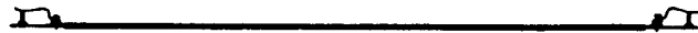
R172 — LINK ASSEMBLY # 3012 CHECK ROD NEW STYLE 6½" PIN/PIN OLD STYLE 6-29/32" PIN/PIN
